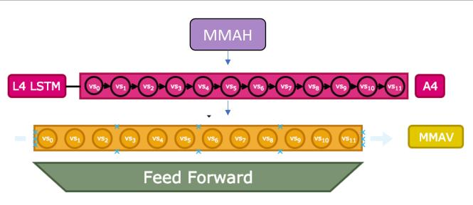
5. We then input the results of the attention to another LSTM layer with the purpose of capturing the relationship of the multiple panoramic images in the route vertically.
